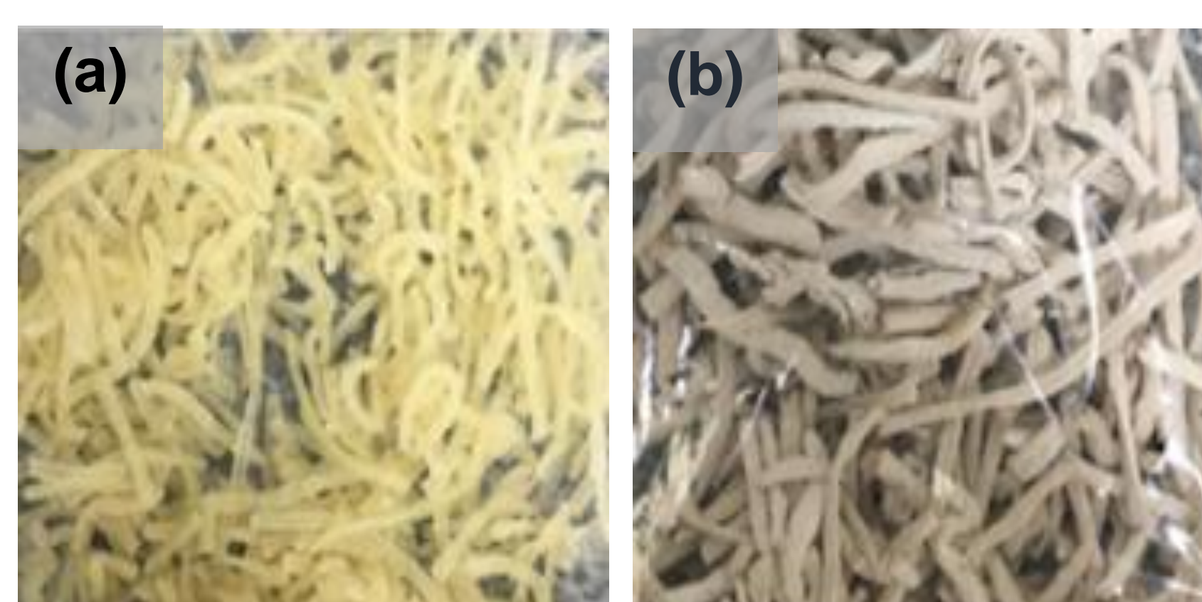
Figure 2. (a) Pure TPS and (b) 75 St_TPS composite, before grinding.
